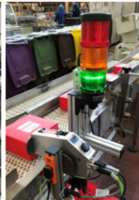
Integra with beacon on conveyor
