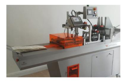
The system comes complete with a full validation package, a reject system and a shingling conveyor to maintain high throughput.
